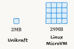
Memory footprint of Unikraft unikernel vs. Linux MicroVMs<sup>1</sup>
